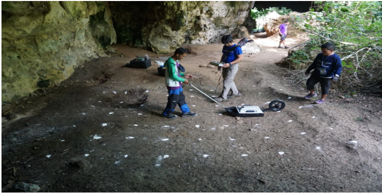
Figure 14. Photo captured during the conducted GPR Survey in the Rock shelter at Tanggapan Cave
