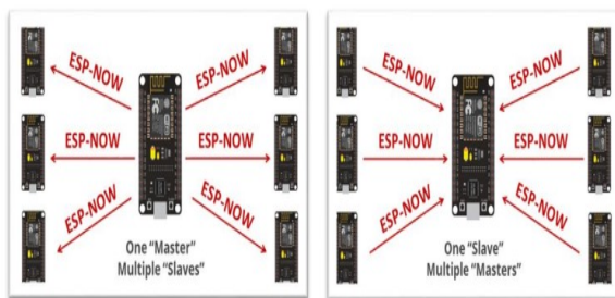
Figure 6. Master-master and Master-slave configuration of the ESP-NOW protocol
