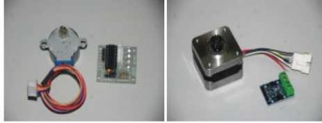
Figure 8 Stepper Motor and H-Bridge Stepper Driver Module(left) and Stepper Motor BYJ48 and ULN2003 Driver Chip(right)
